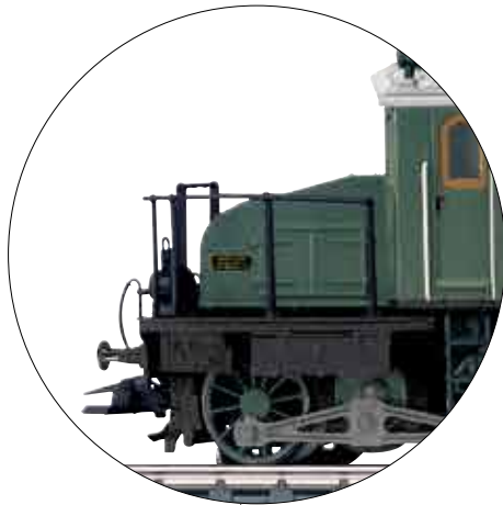
Drive system prototypically be means of a jackshaft
