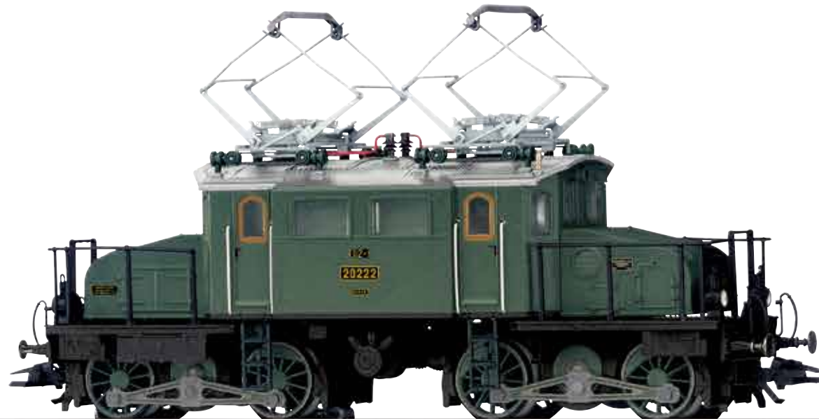
Drive system prototypically be means of a jackshaft
